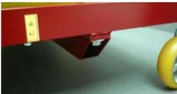
The contact pins for potential equalisation are to be found beneath the chassis. Their position is marked with a yellow, rectangular sticker on a vertical surface next to them.
