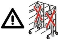
Do not climb on the rack! Do not ride on the rack! The Transport Rack has not been designed to climb on, to travel with, or to transport people. This may overload the rack and cause it to tip over. The Transport Rack has been exclusively designed to hold and transport materials.
